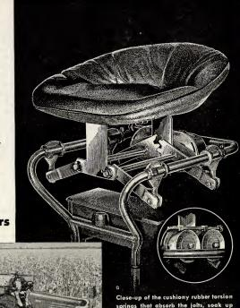
springs that absorb the jolts, soak up shocks and level out rough rebounds. The new Ridemaster seat is adjustable,
